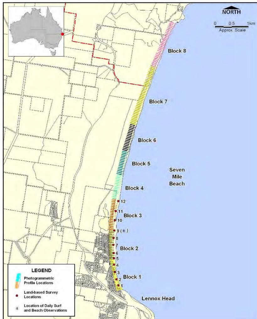
Illustration 3.3 - Proposed Land-based Surveys and Photogrammetry Sections – Lennox Head
