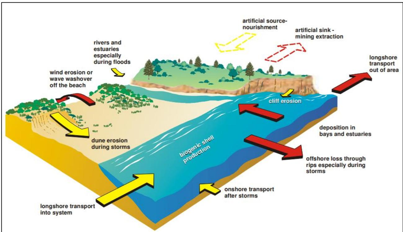
**FIGURE 3-5 MODEL SEDIMENT COMPARTMENT SHOWING POTENTIAL SEDIMENT INPUTS AND LOSSES (NSW DEPARTMENT OF LAND AND WATER CONSERVATION)**
