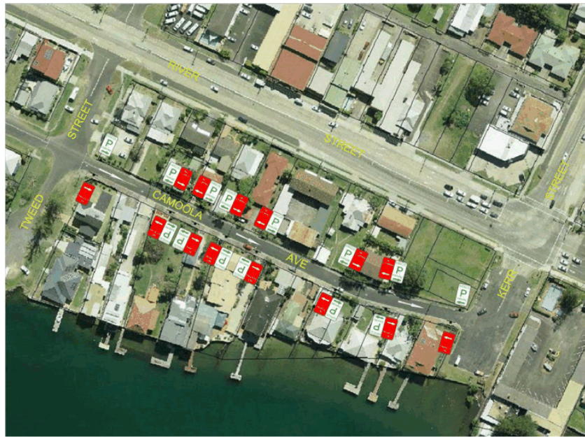
Option 5 - Camoola Avenue, One Way Traffic Eastward - Staggered Parking Both Sides
