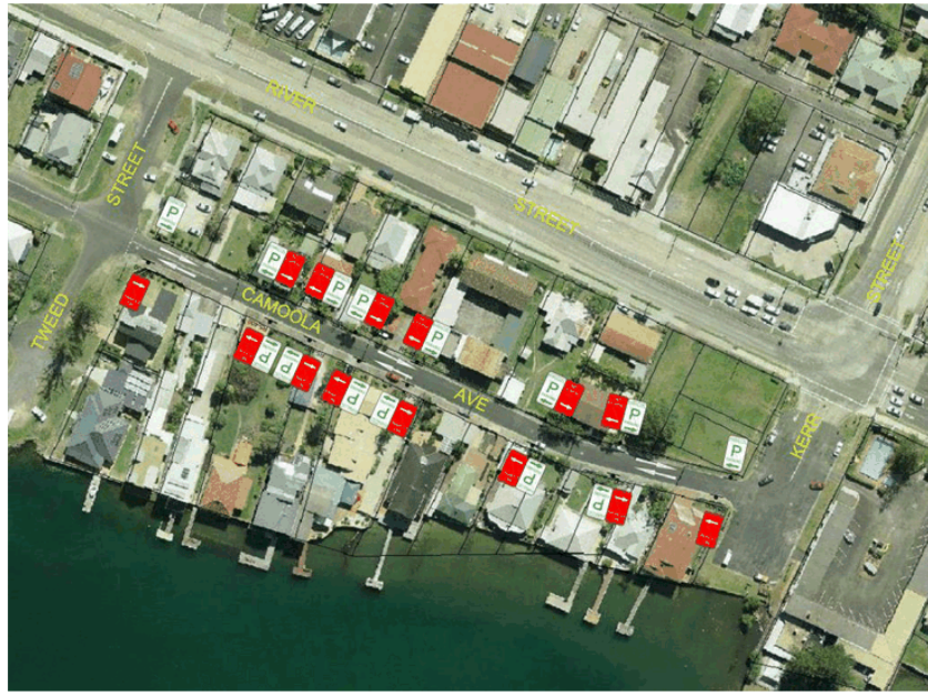
Option 4 - Camoola Avenue, Two Way Traffic - Staggered Parking Both Sides
