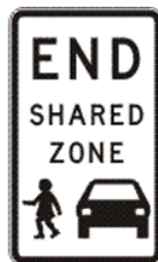
FIGURE 4: END SHARED ZONE TRAFFIC SIGN R 4-5
