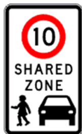
FIGURE 3: START SHARED ZONE TRAFFIC SIGN R 4-4
