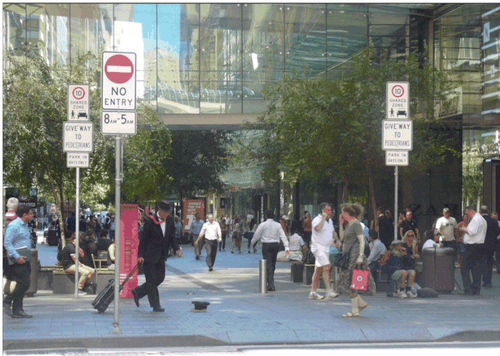
Figure 1. Photo and diagram of a Category 1 shared zone showing regulatory signage, typical layout and treatments. [Note: The No Entry sign is site specific] The photo may have been modified to demonstrate essential elements.
