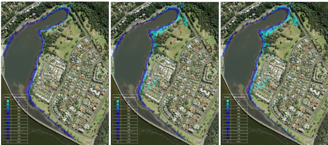
Figure 20: Predicted present day inundation due to 1, 50 and 100 year ARI ocean level events (not including wave setup)
