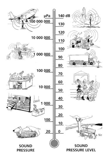
Our hearing covers a wide range of sound pressures – a ratio of over a million to one. The dB scale makes the numbers manageable.
