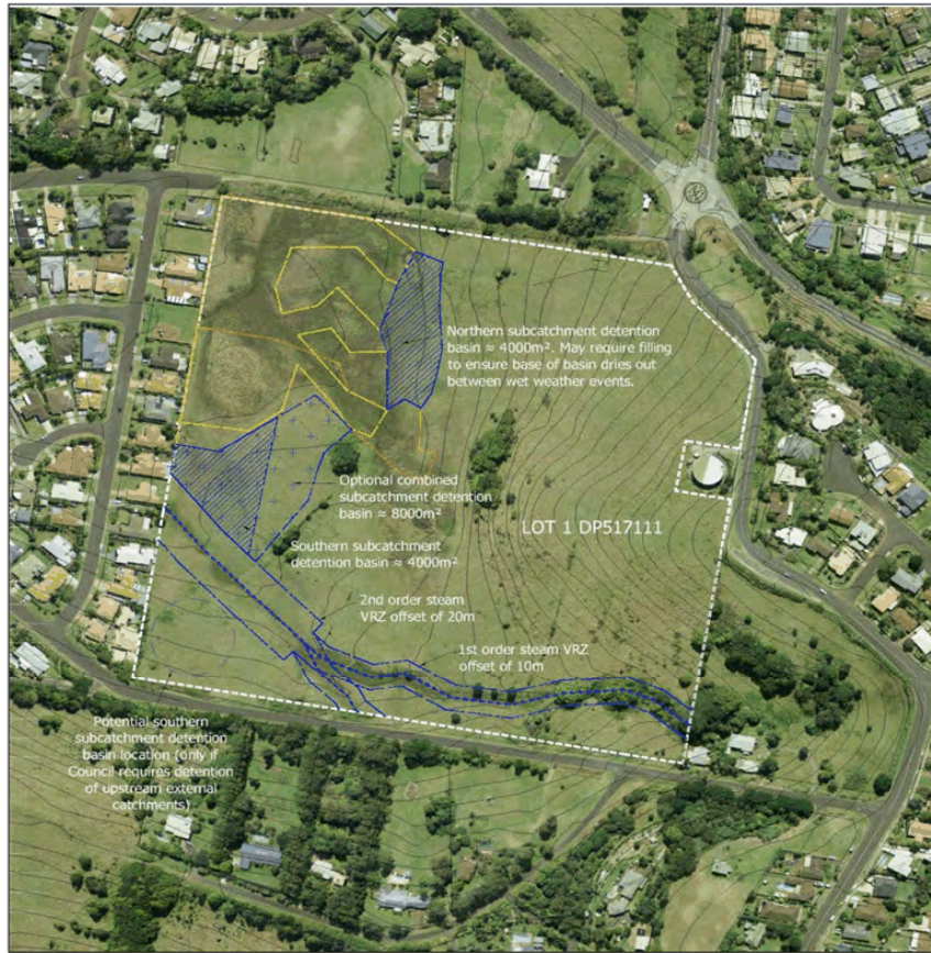
Figure 6: Approximate location of stormwater detention areas to be retained in RU1 zone
