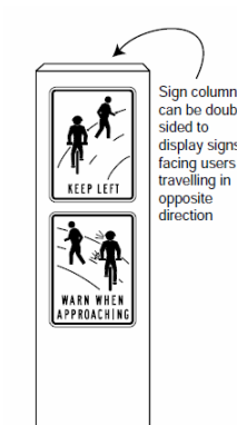
(f) Level 2 sign column
