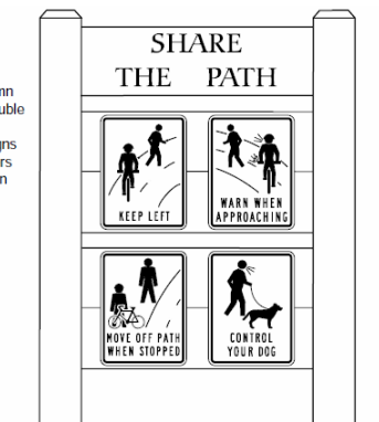
(g) Alternate layout of group sign for where space is limited
