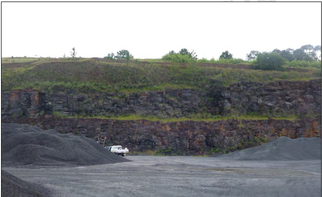
Plate 9 East Wall Weathering Profile at Tuckombil Quarry The thickness of overburden being the chief issue for further development in this orientation.
