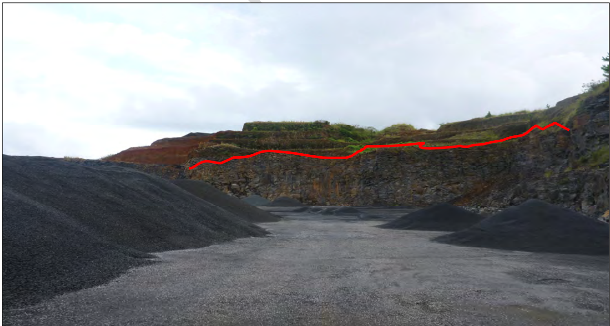
Plate 8 North Wall Weathering Profile at Tuckombil Quarry Red line denoting the transition from distinctly weathered material to unweathered basalt. This photograph also shows the rapidly thickening overburden sequence which develops to the north of site.
