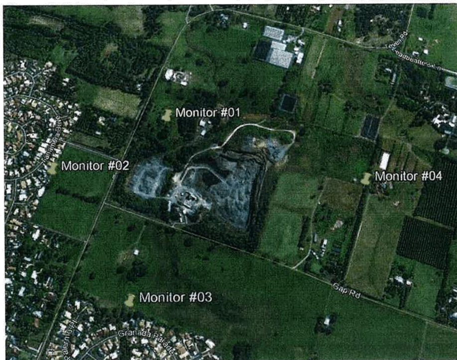
Figure 2: An overview of the quarry location with respect to blast monitor locations.
