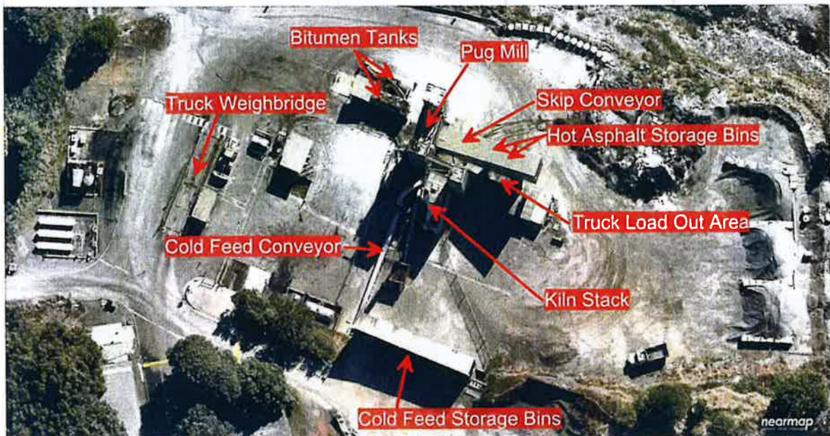
Figure 3-2 Alstonville plant process components and emission sources
