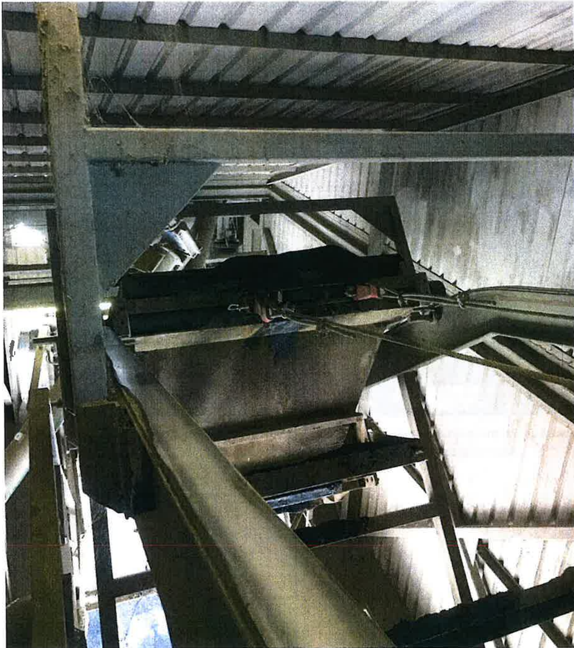
Figure 3-4 The loaded asphalt skip moving up the conveyor towards the Hot Asphalt Storage Bins
