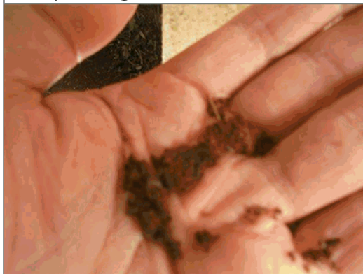
23: Surface soils are low plasticity silty clays (CL) with trace of sand
