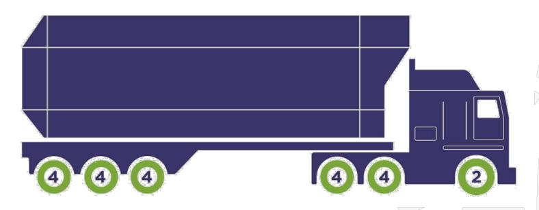
Since the introduction of SCHMS and strong commitment from Sunshine Sugar, axle mass compliance has improved significantly and average bin masses have reached **22.01 tonnes**. Mass monitoring equipment fitted to vehicles and load management procedures by Sunshine Sugar have delivered significant pavement and safety outcomes for the community.
