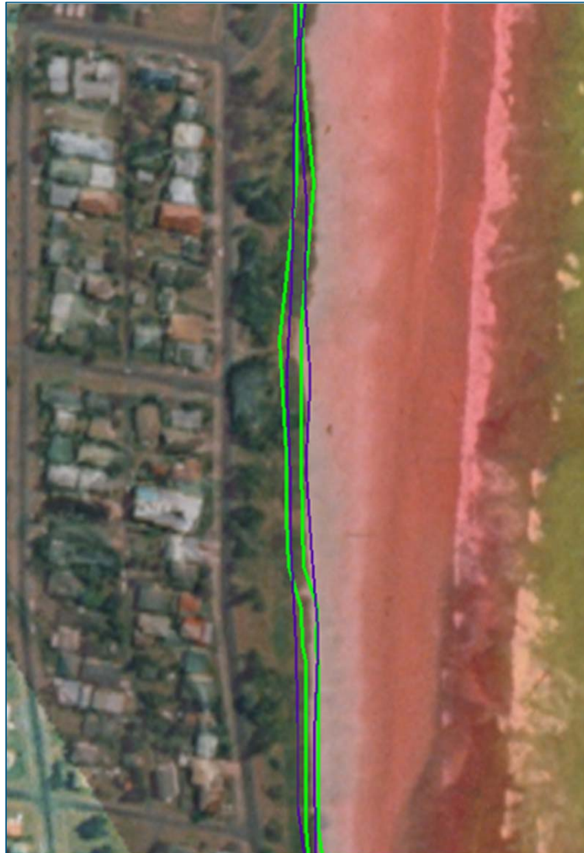
Figure 4-4 Comparison of GPR predicted rock seawall (blue) and 1967 scarp line
