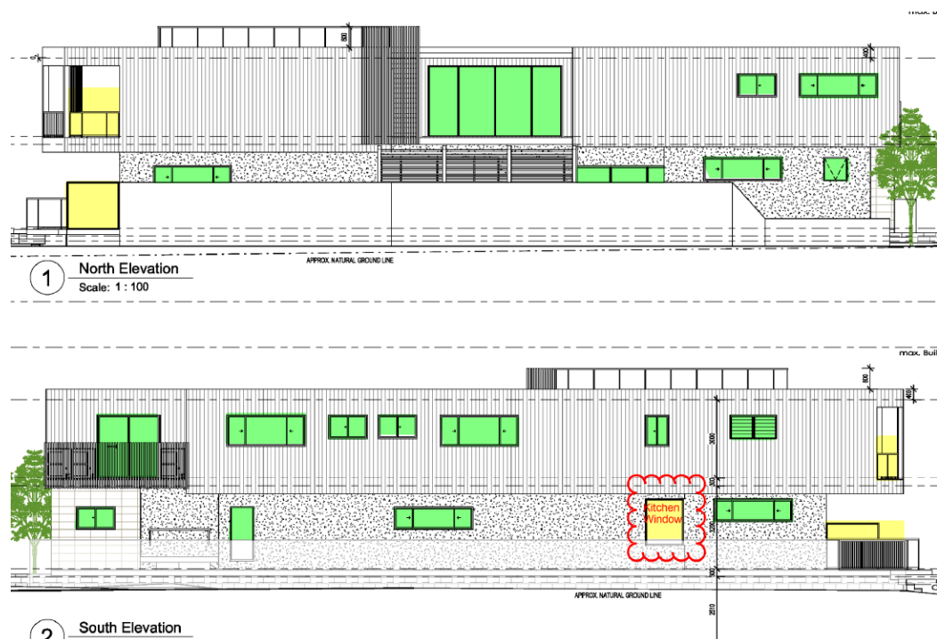
Figure 5: Privacy assessment – kitchen window highlighted
