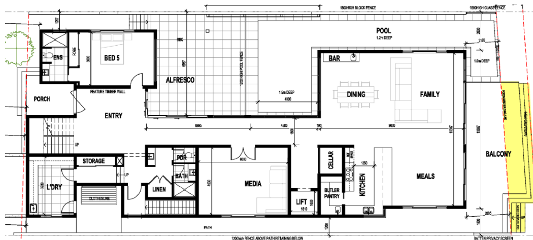
Figure 6: Ground floor encroachment in to foreshore building line
