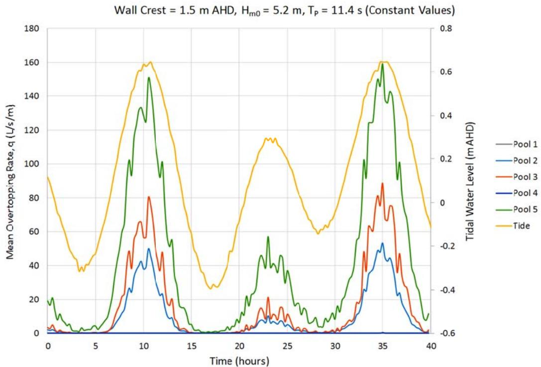
**Figure 7.7** Overtopping Ballina pool positions 1 year ARI waves, wall at 1.5 m AHD
