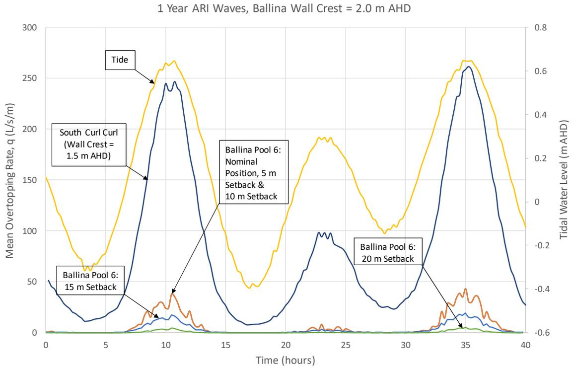
**Figure 9.7** Overtopping for Pool position 3 (wall at 2.0 m AHD), 1 year ARI waves
