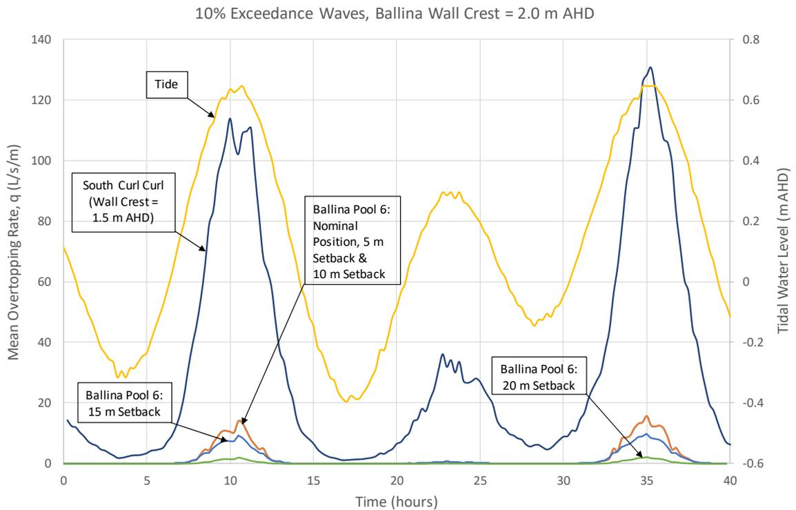
**Figure 9.6 Overtopping for Pool position 3 (wall at 2.0 m AHD), 10% exceedance waves**
