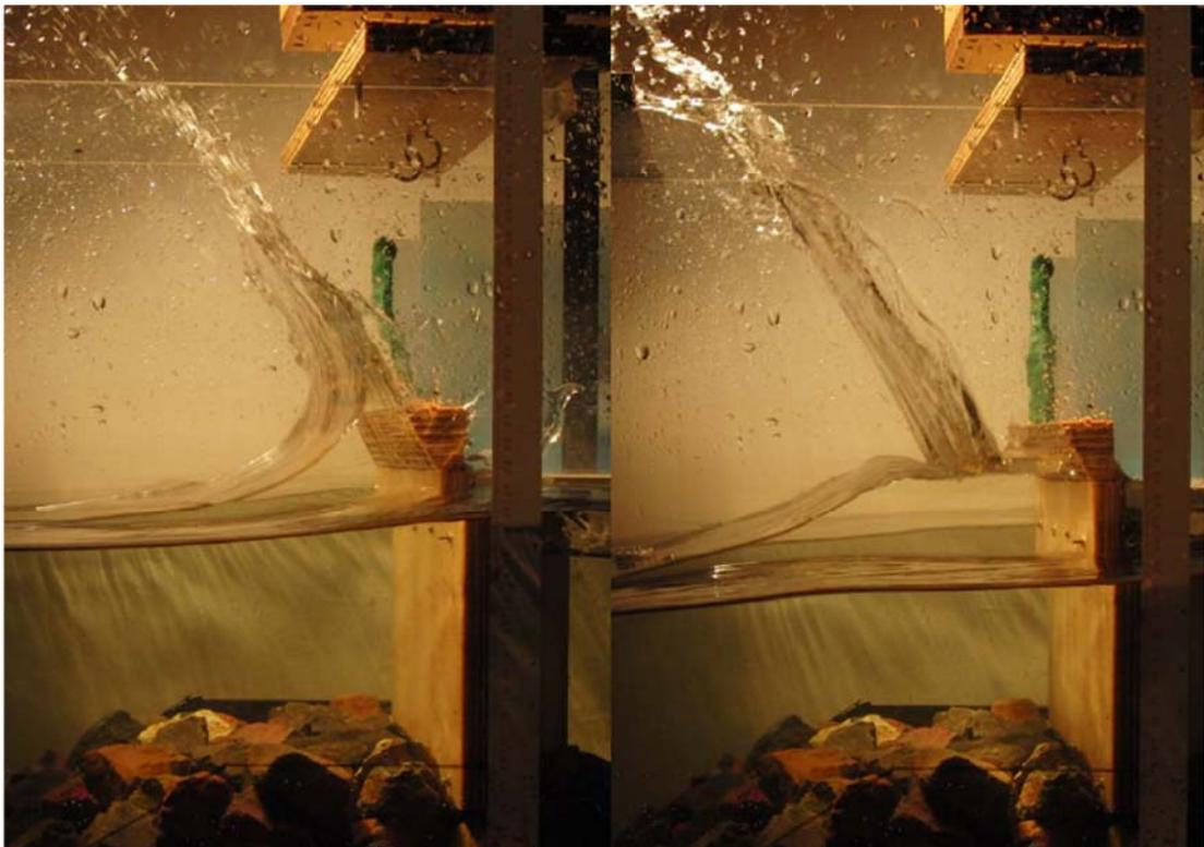
**Figure 6.3 Angled wave deflector wall physical model**
