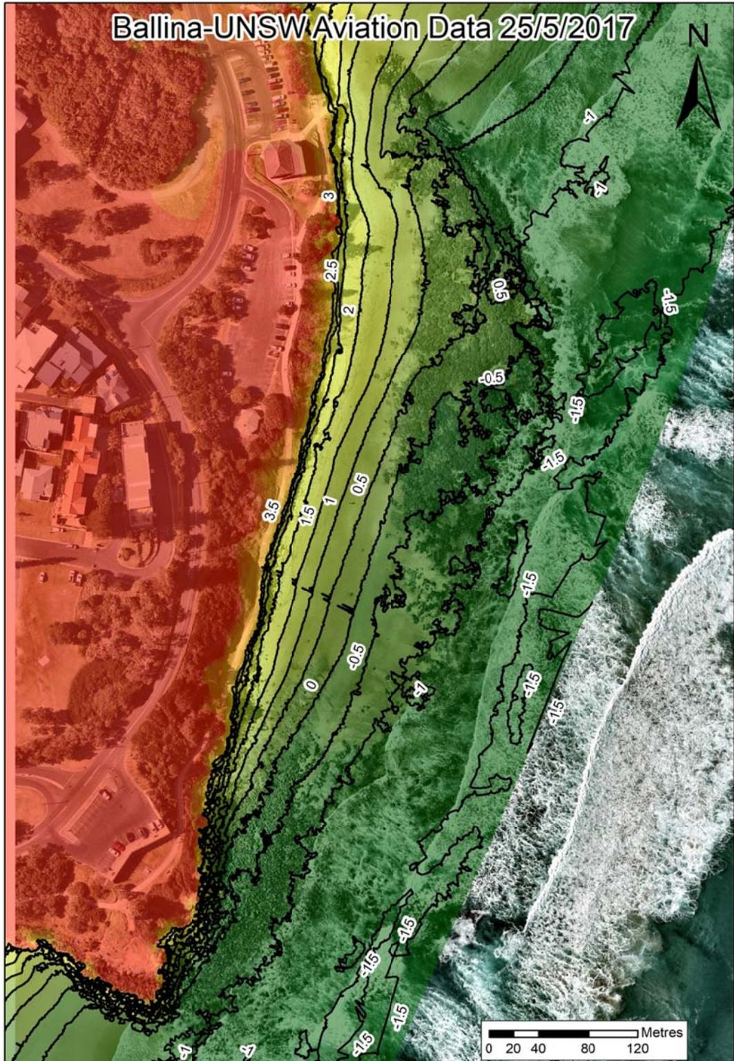
Figure 7.2 UNSW LIDAR survey data transformed into contours
