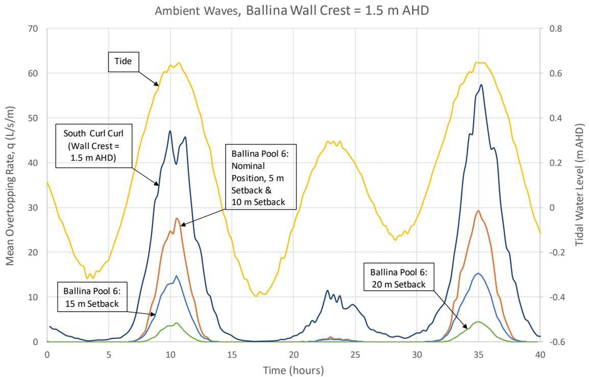
**Figure 9.2 Overtopping for Pool position 3 (wall at 1.5 m AHD), ambient waves**
