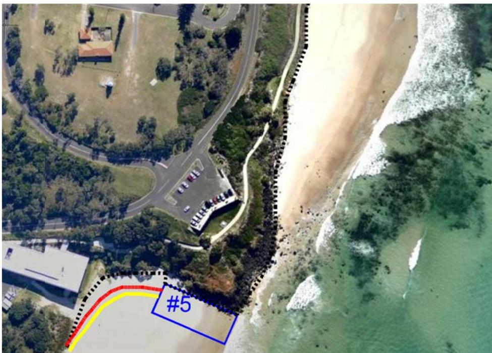
Notes: Black dashed line is present 2 m AHD contour based on optical drone survey by WRL on 8/8/2018;
