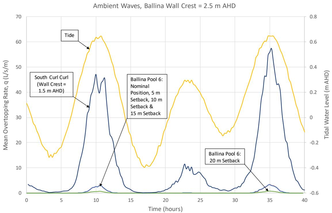
**Figure 9.8** Overtopping for Pool position 3 (wall at 2.5 m AHD), ambient waves
