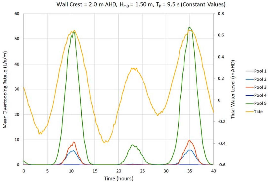
**Figure 7.8** Overtopping Ballina pool positions ambient waves, wall at 2.0 m AHD
