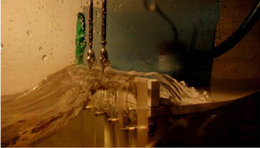
**Figure 6.2 Wave overtopping physical model**
