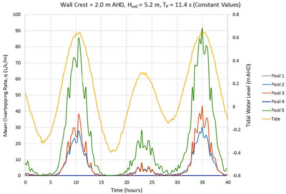
**Figure 7.10** Overtopping Ballina pool positions 1 year ARI waves, wall at 2.0 m AHD
