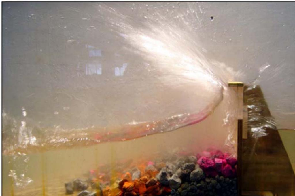
**Figure 6.4 Curved wave deflector wall physical model**
