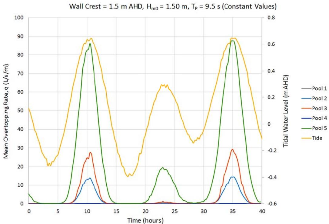
Figure 7.5 Overtopping Ballina pool positions ambient waves, wall at 1.5 m AHD
