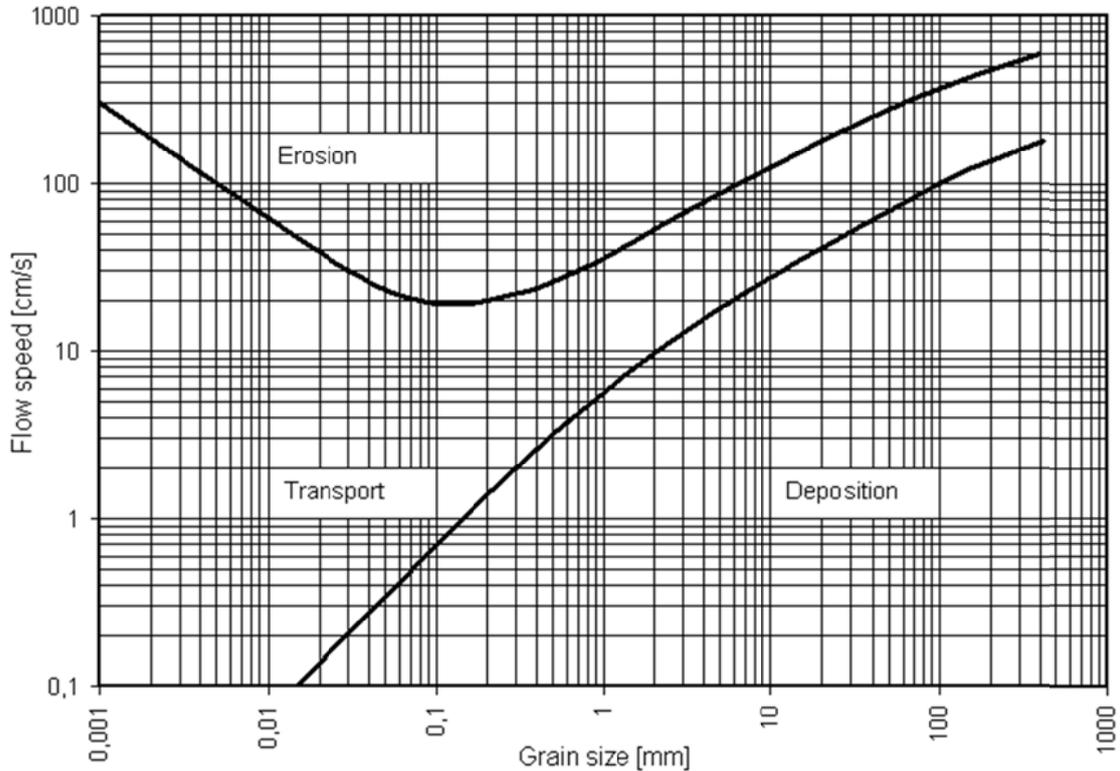
**Figure 5.7 Hjulstrom diagram for sand erosion**
