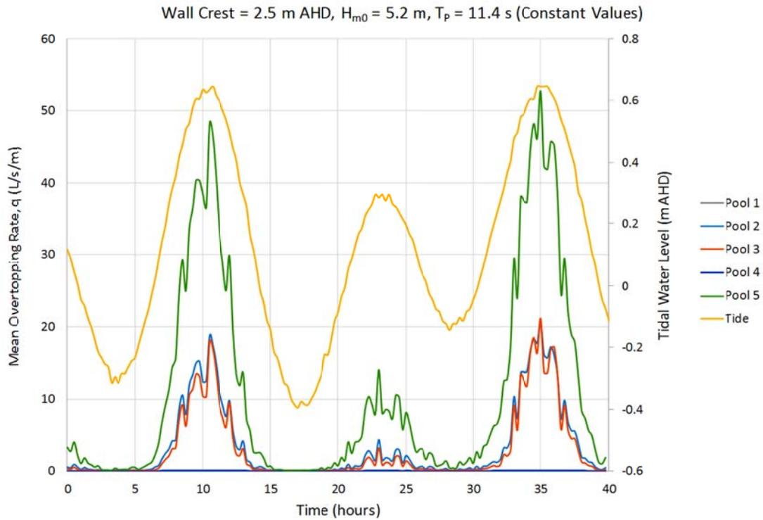
**Figure 7.13** Overtopping Ballina pool positions 1 year ARI waves, wall at 2.5 m AHD
