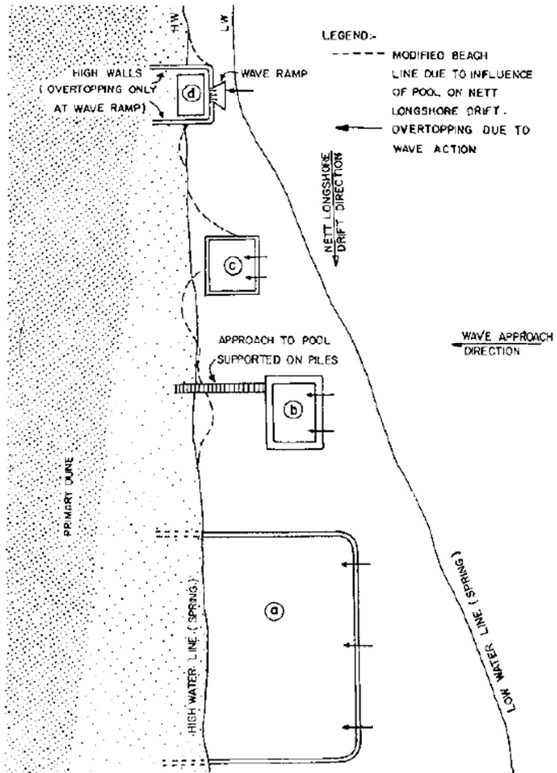
Figure 2.1 Schematisation of pools (Figure 3 of Bosman and Scholtz, 1982)
