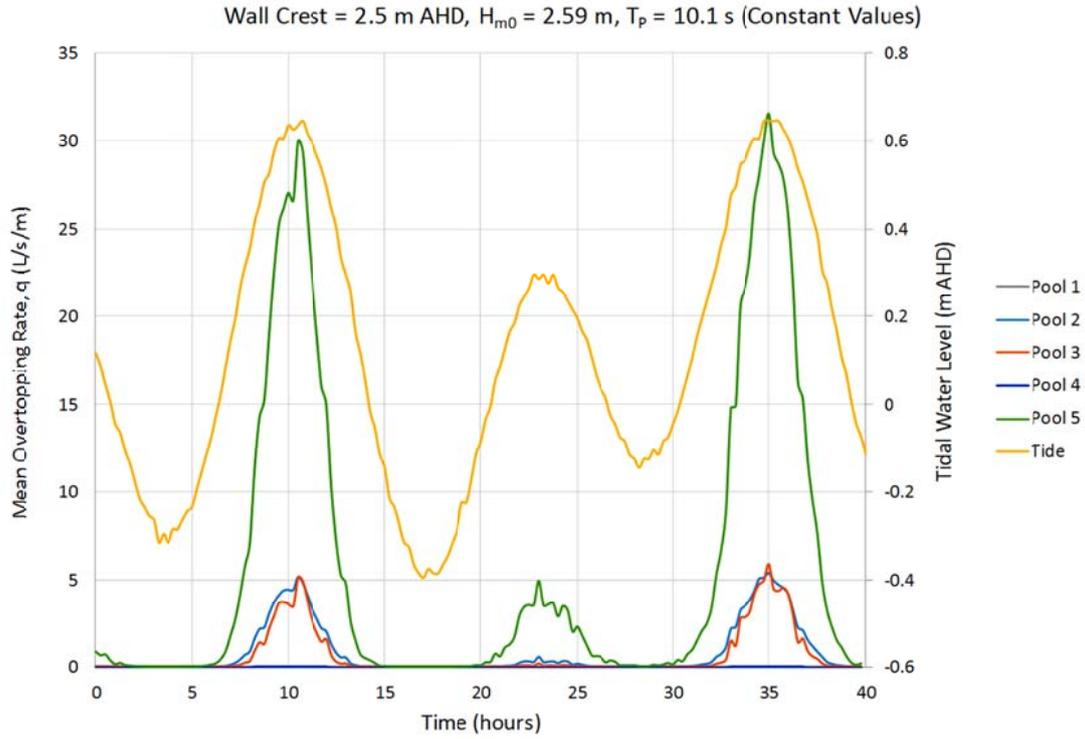
**Figure 7.12** Overtopping Ballina pool positions 10% exceedance waves, wall at 2.5 m AHD
