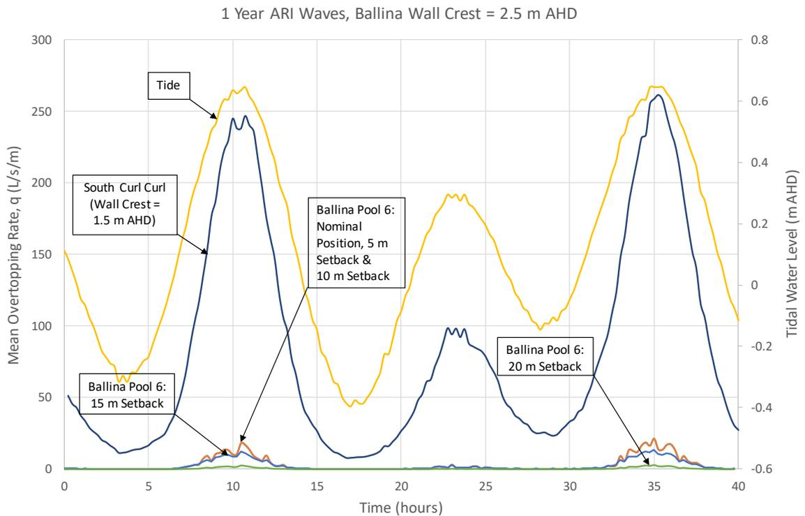
**Figure 9.10 Overtopping for Pool position 3 (wall at 2.5 m AHD), 1 year ARI waves**
