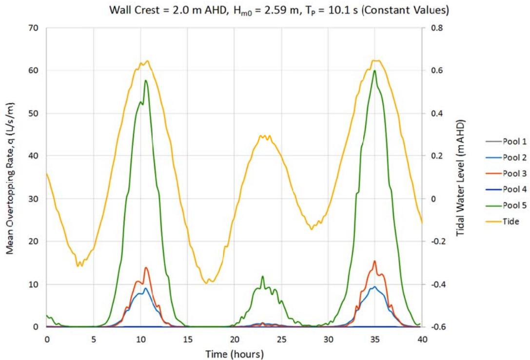
**Figure 7.9** Overtopping Ballina pool positions 10% exceedance waves, wall at 2.0 m AHD
