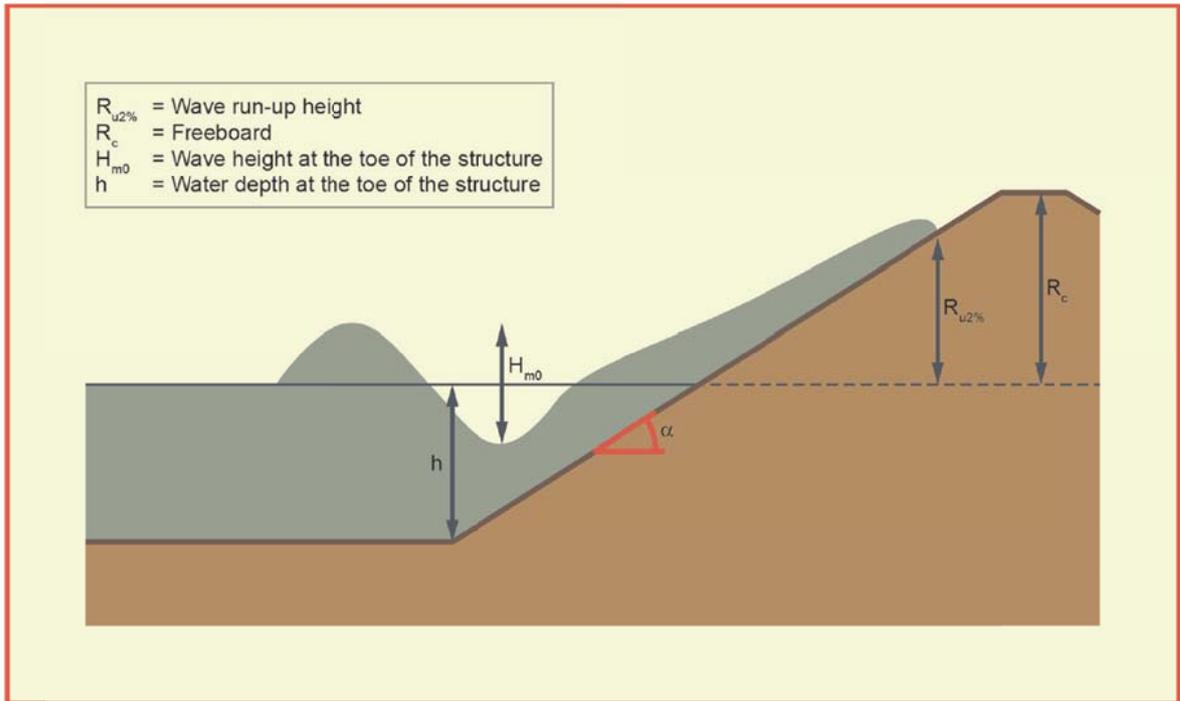
Figure 6.1 EurOtop cross section for overtopping
