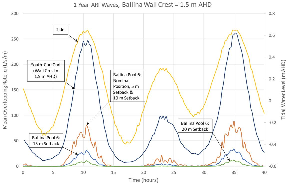
**Figure 9.4 Overtopping for Pool position 3 (wall at 1.5 m AHD), 1 year ARI waves**
