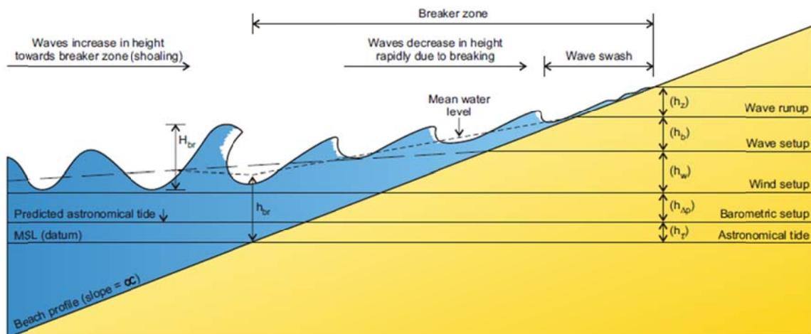
Figure 4.1 Components of elevated water levels (Adapted from NSW DECCW, 2010)
