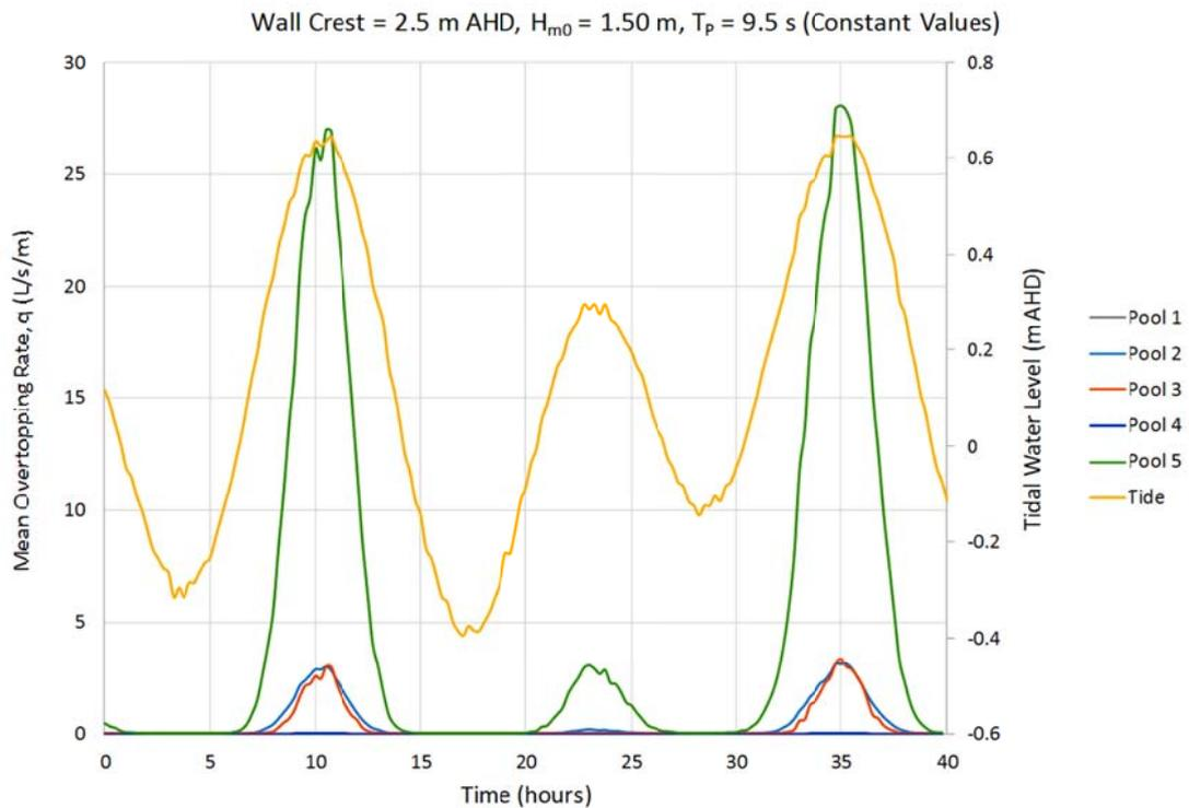
**Figure 7.11** Overtopping Ballina pool positions ambient waves, wall at 2.5 m AHD
