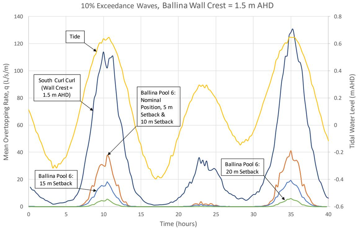
**Figure 9.3 Overtopping for Pool position 3 (wall at 1.5 m AHD), 10% exceedance waves**
