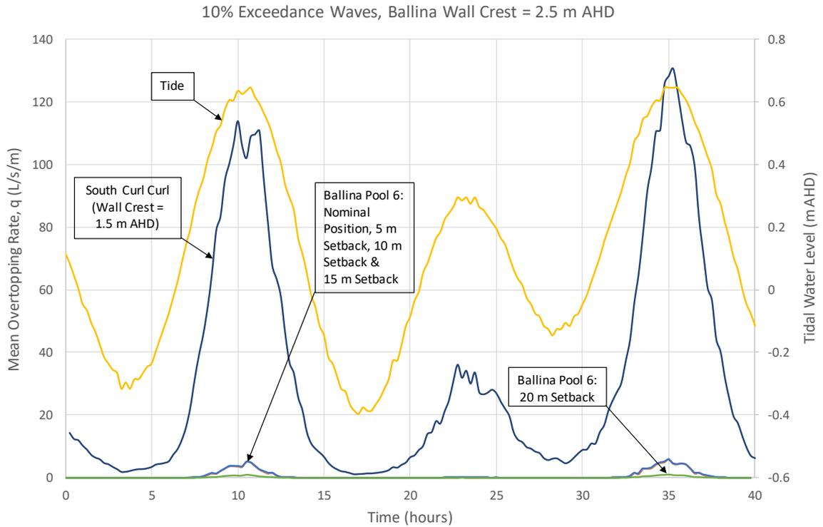
**Figure 9.9 Overtopping for Pool position 3 (wall at 2.5 m AHD), 10% exceedance waves**
