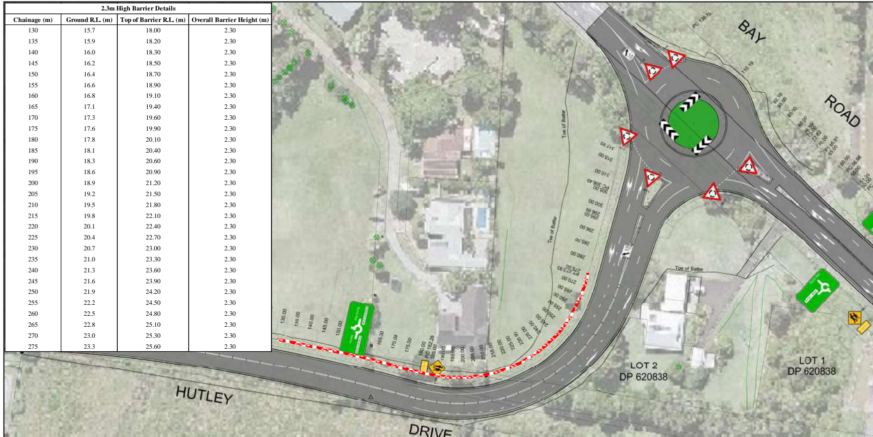
Sketch No. 2: Road Extension Layout and 2.3m High Acoustic Barrier Scenario (Not to Scale).
