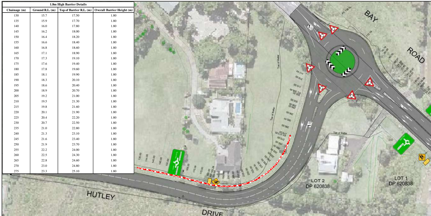
Sketch No. 1: Road Extension Layout and 1.8m High Acoustic Barrier Scenario (Not to Scale).
