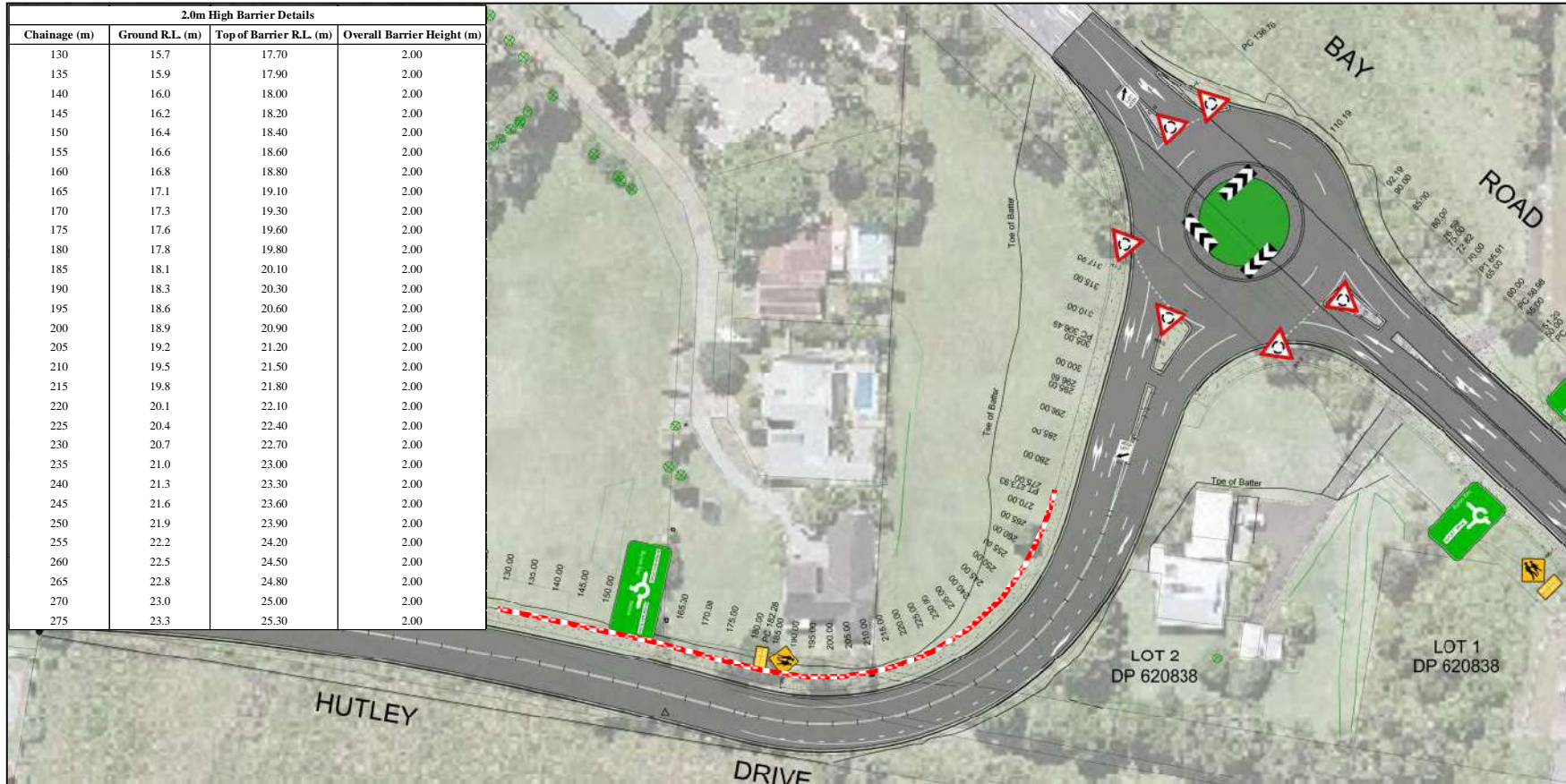
Sketch No. 3: Road Extension Layout and 2.0m High Acoustic Barrier with OGA or SMA Road Surface Scenario (Not to Scale).
