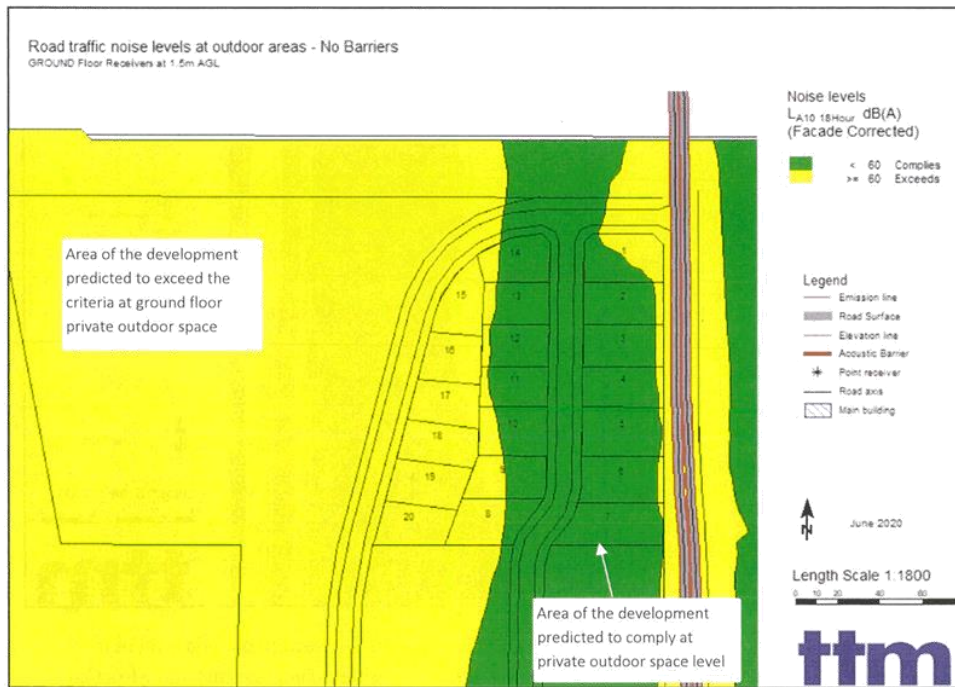
Figure 4: Predicted Ground Floor Private Outdoor Space Road Traffic Noise Levels – No Acoustic Barriers
