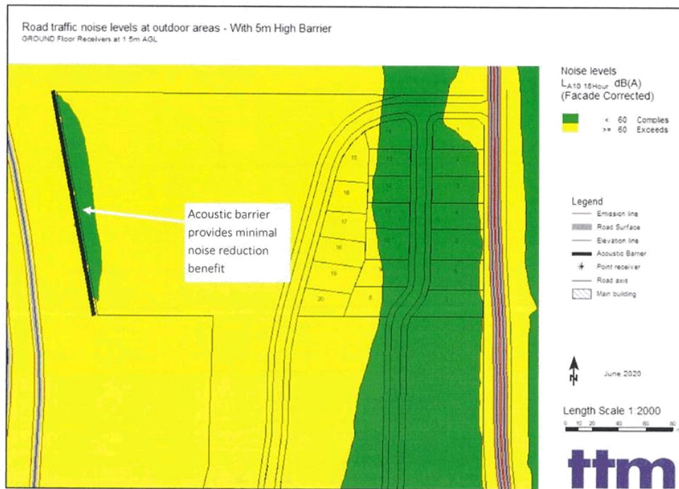
Figure 5: Predicted Ground Floor Private Outdoor Space Road Traffic Noise Levels – With Acoustic Barriers
