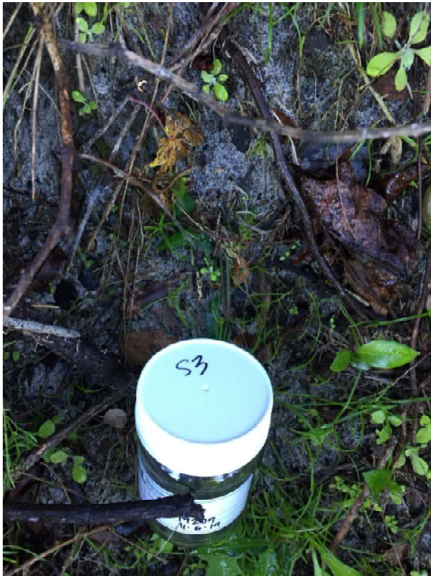
Image 6: An image of where sample 'S3' was collected in the understorey of the rear yard, the fine dune sand is visible beneath the vegetation
