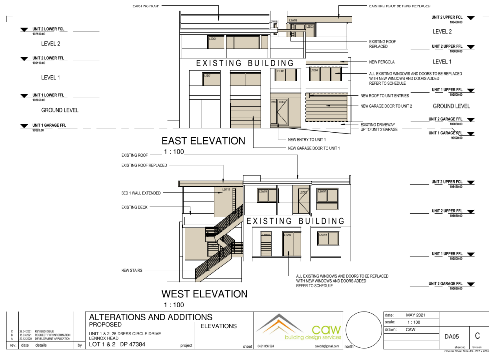
Figure 5: East and West Elevations
