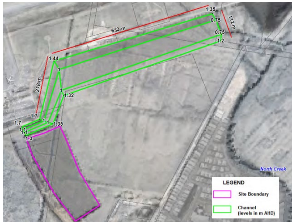
Figure 2 – Conceptual Design of Mitigation Channel (BMT)
