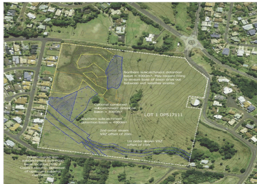
Plate 2: Extract from rezoning documentation confirming stormwater basins should be located outside of known threatened species habitat. The yellow lines represent known ecological constraints.
