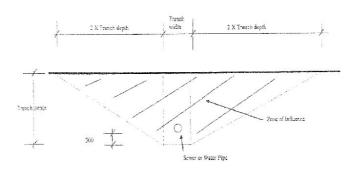
The "Zone of Influence" extends out from the edge of the asset/pipe trench twice the distance as the depth of the trench. (The ratio used is 2:1). For sand, filled ground (including controlled fill), loam, etc, the zone will extend twice the depth of the trench plus half the width of the trench –
