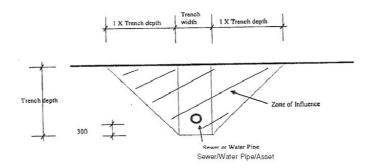
The "Zone of Influence" extends out from the edge of the asset/pipe trench the same distance as the depth of the trench (The ratio used is 1:1). For clay soils the zone will extend the same distance as the depth plus half the width of the trench each side of the asset:
