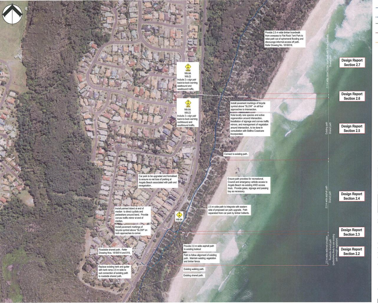
Proposed shared path (asphalt surface, width as shown)
