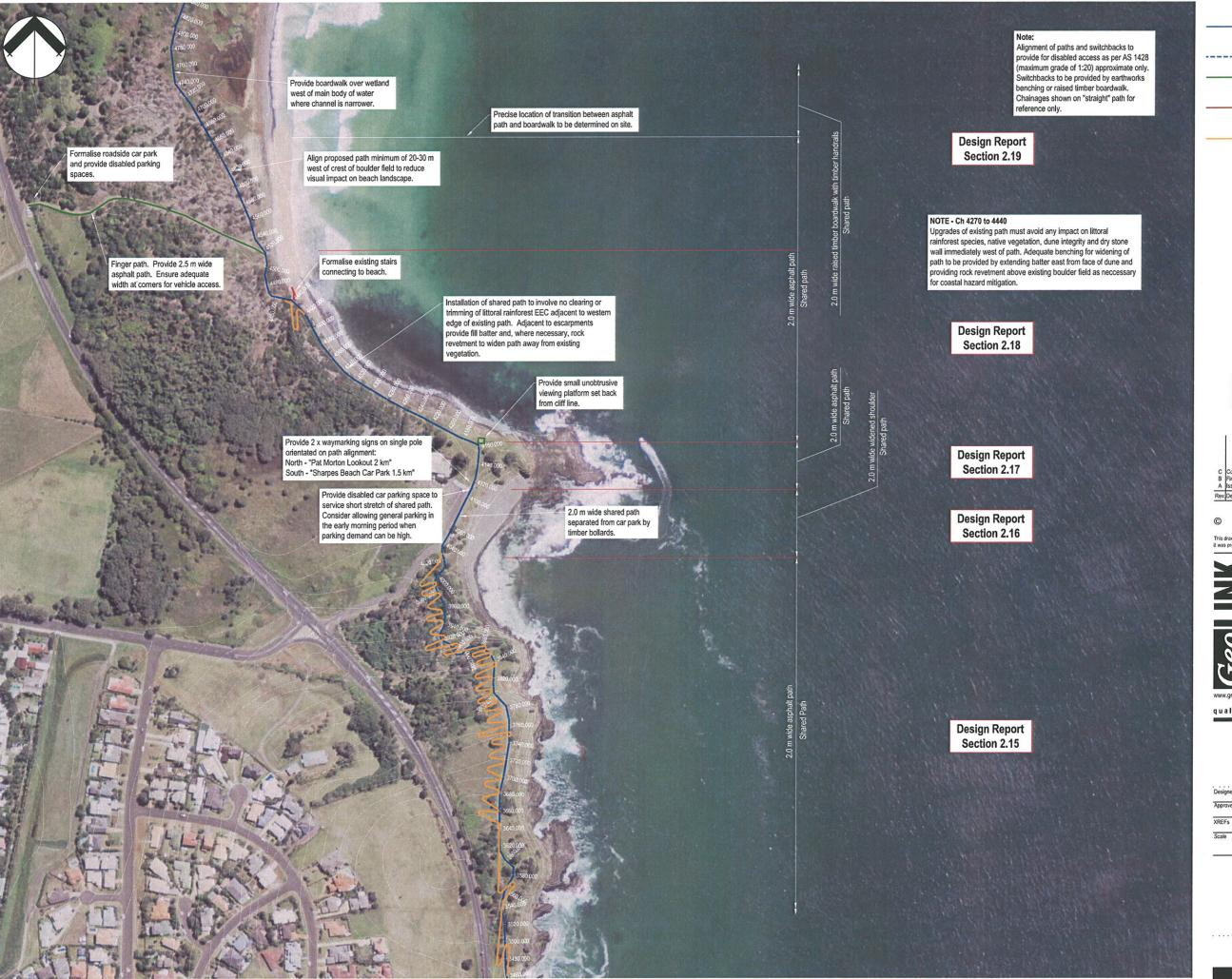
Proposed shared path (asphalt surface, width as shown)
