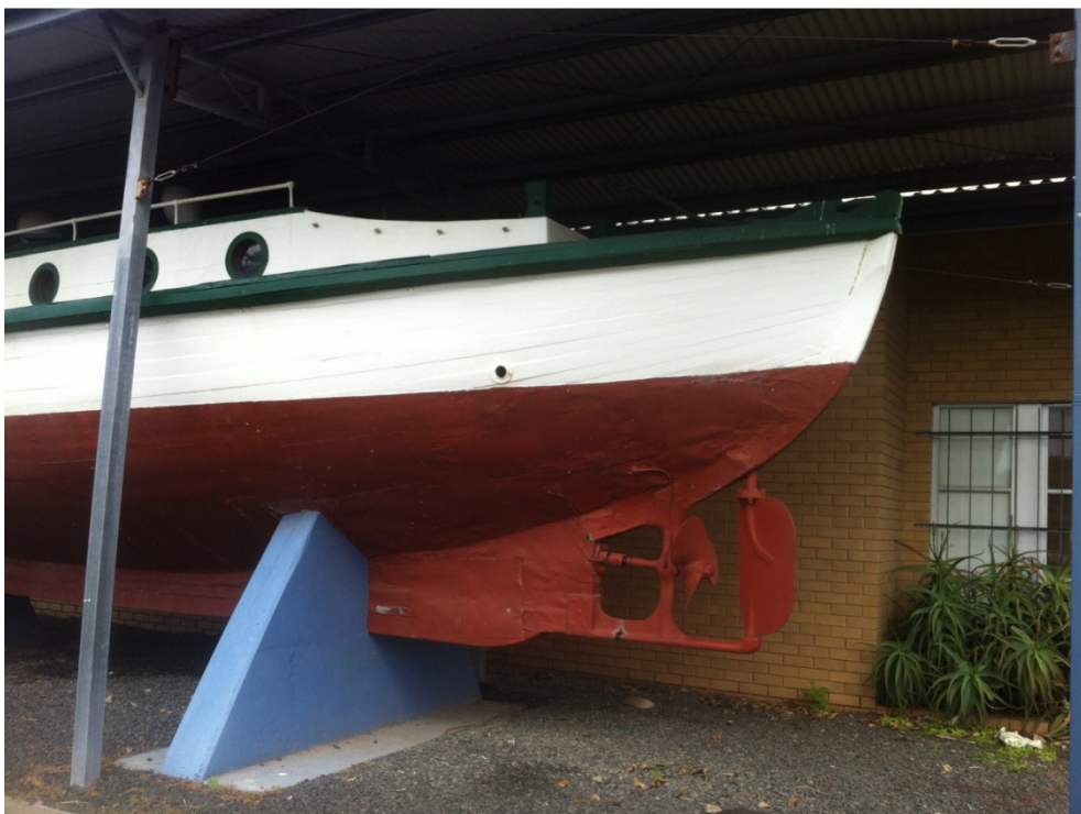
Plate 12: PV Richmond looking toward the stern. Note hull intrusive tin-alloy sheathing repairs are coming away from the hull. Not also that gap beginning to form between the keel and keelson (March 2012).
