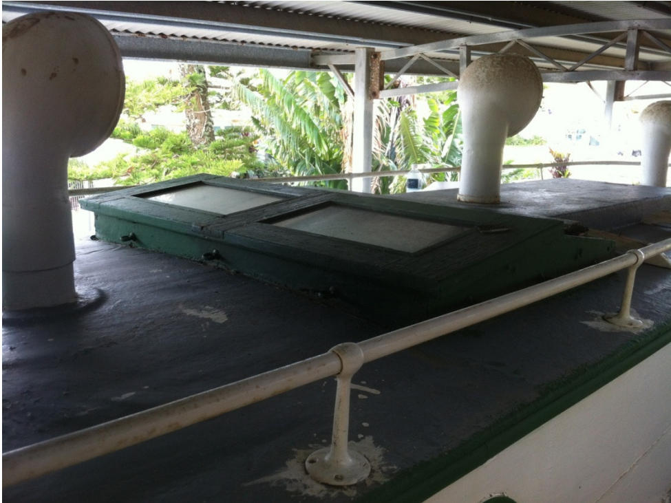
Plate 15: PV Richmond looking across cabin roof. Note intrusive grey fibreglass coating and damage to cabin roof timbers/hatch covers (March 2012).
