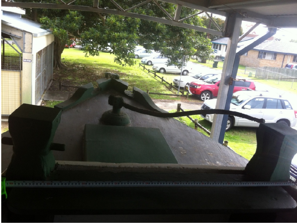
Plate 17: PV Richmond looking across stern. Note tiller in foreground and poor state of deck sheathing (March 2012).
