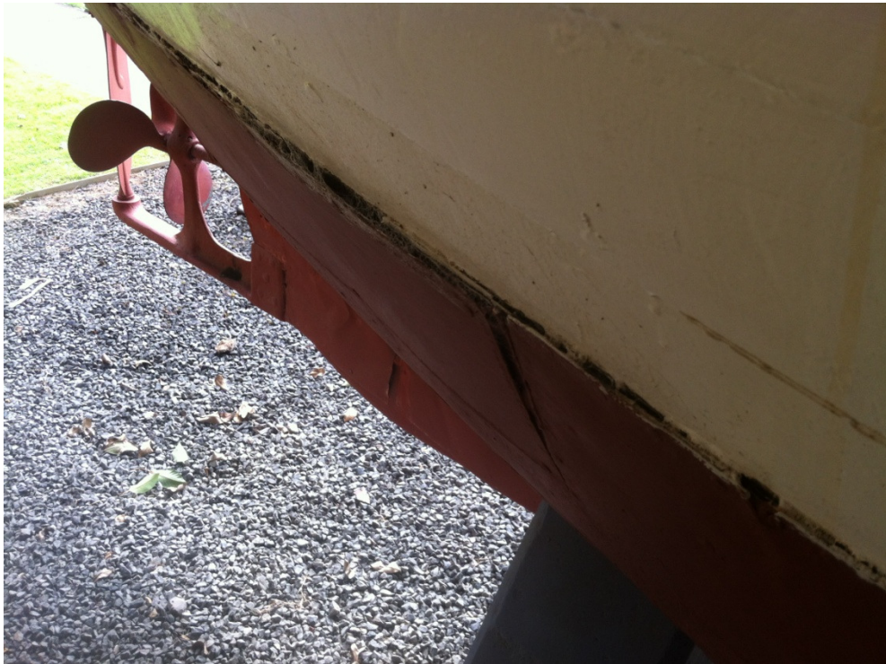
Plate 13: PV Richmond looking toward the stern. Note hull intrusive tin-alloy sheathing repairs are coming away from the hull. (March 2012).
