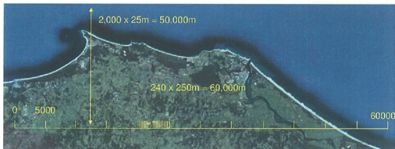
Figure 8: Model extent and grid element representation
