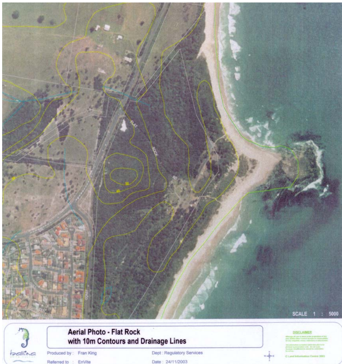
Figure 5: Aerial photo of the northern section of the study site showing contours (yellow) and drainage lines (blue). Flat Rock can be seen in the lower half of the photo (Ballina Shire Council, 2003).
