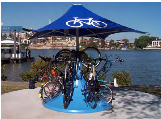
Figure 13. Radial vertical bicycle parking
