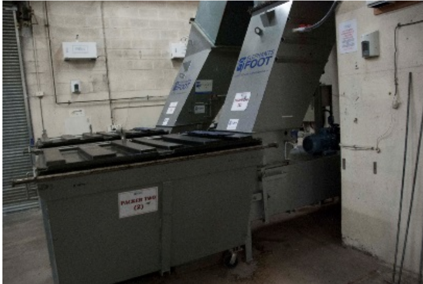
Two x 3 m 3 bulk bins attached to a small-scale static compactor at the base of a chute (Photo: Andrew Quinn)
