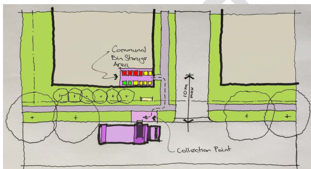
Figure 11 Communal bin storage area for bulk or mobile bins and on-site collections (EPA note on this figure: this is an original figure that will require revamping)
