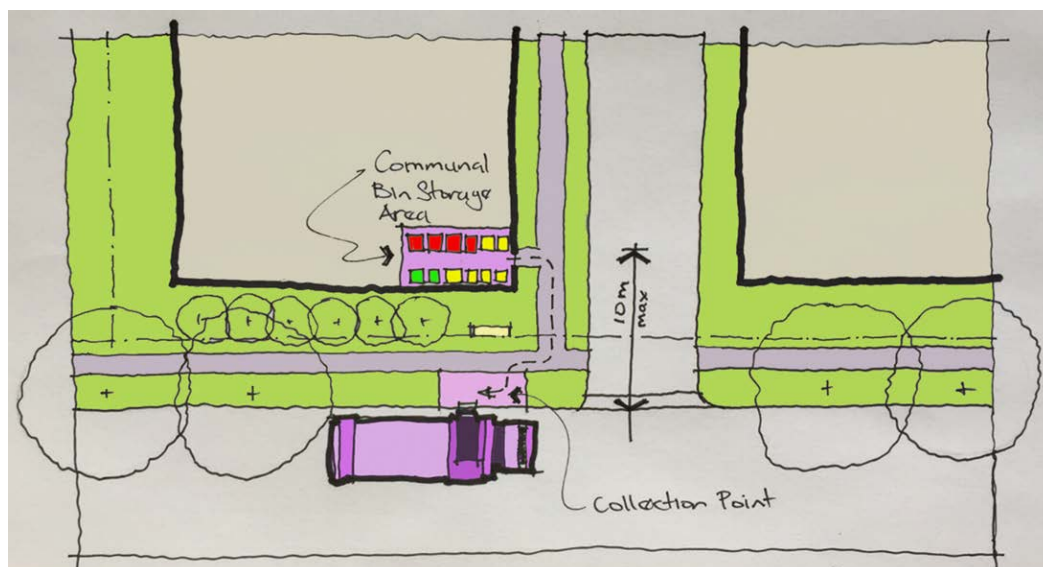
Figure 8 Example of a communal storage area for bulk bins or mobile bins and on-site collections
