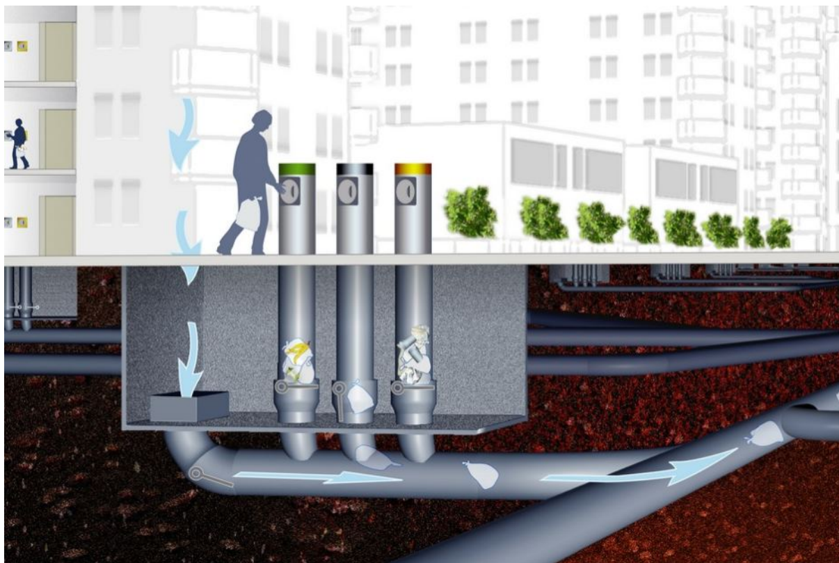
Automated waste collection system (Photo: Envac Australia)
