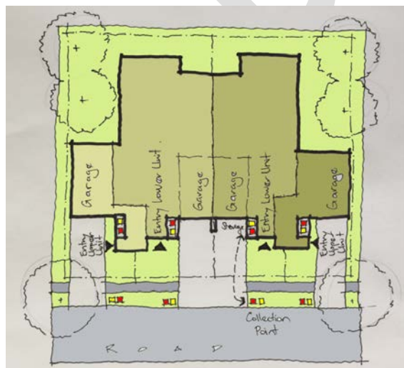
Figure 4 and Figure 5 Individual bin storage areas provided for each attached dwelling (EPA notes that these are new figures that needs to be designed)
