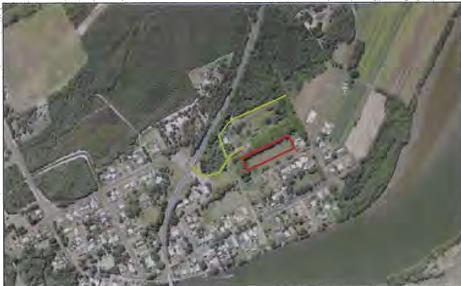
Figure 8— Driveway and road providing fire brigade access to the hazard vegetation.
