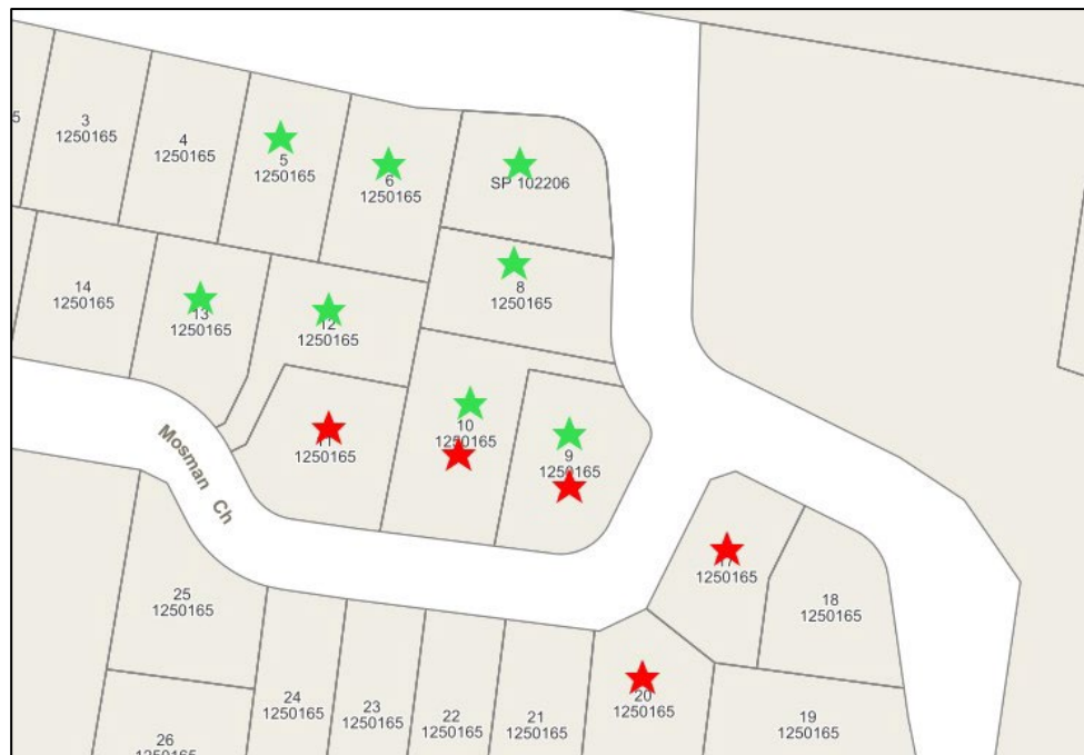
Figure 2: Lots burdened and benefited – S.88B instrument (red stars indicate lots burdened, green stars indicate lots benefited).
