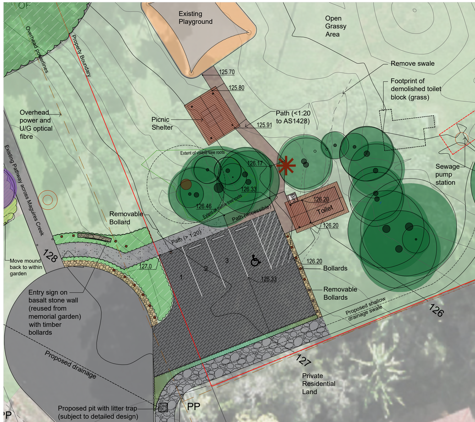
Aerial Photo Reference: NSW Spatial Services 2021 Scale at A3 1:200 Contours represent the site levels at the time of survey. This is a conceptual plan only and is subject to detailed design. Design levels shown are approximate only.
