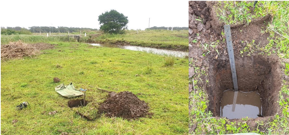
Figure A.22: Pit used to measure hydraulic conductivity adjacent to KH_P2
