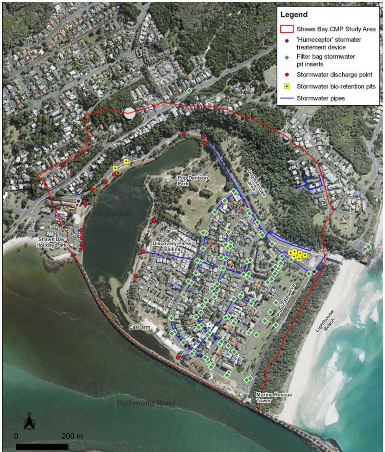
Figure 22: Shaws Bay stormwater infrastructure
