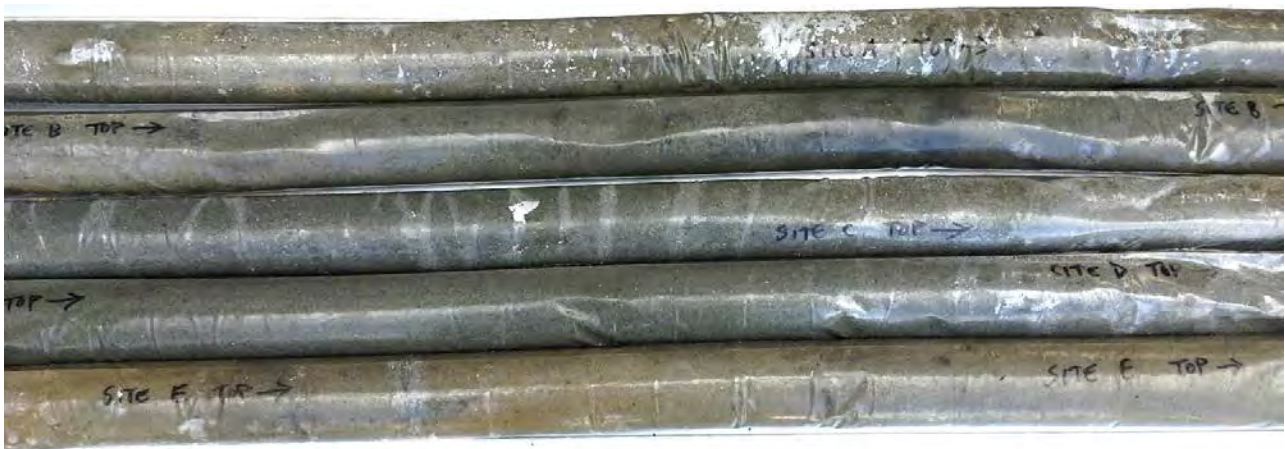
Figure 2: Extracted cores within plastic liners prior to splitting and core logging
