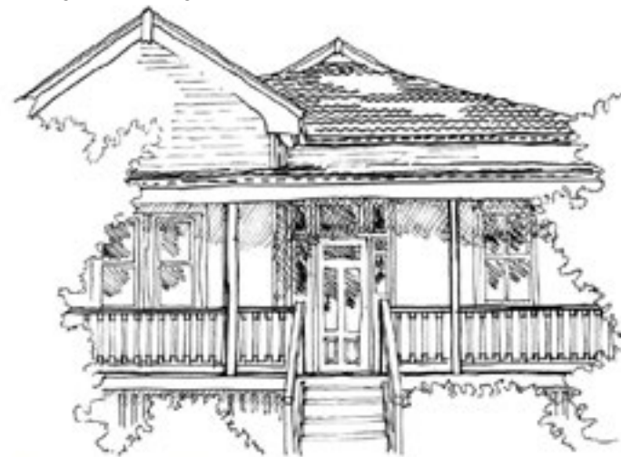
Figure C1.3 – Roof replacement – tiling The use of concrete and terra cotta roofing tiles on buildings in place of corrugated steel or AC roof sheeting is usually not appropriate due to the heavy loads imposed on the lightweight roof framing by the tiles. Tiles also look too heavy in most instances when used on weatherboard buildings with lightweight elements such as verandahs and window hoods.
