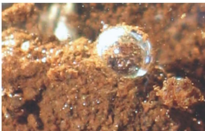
Figure 1. An air bubble escaping from an air-dry aggregate submerged in water
