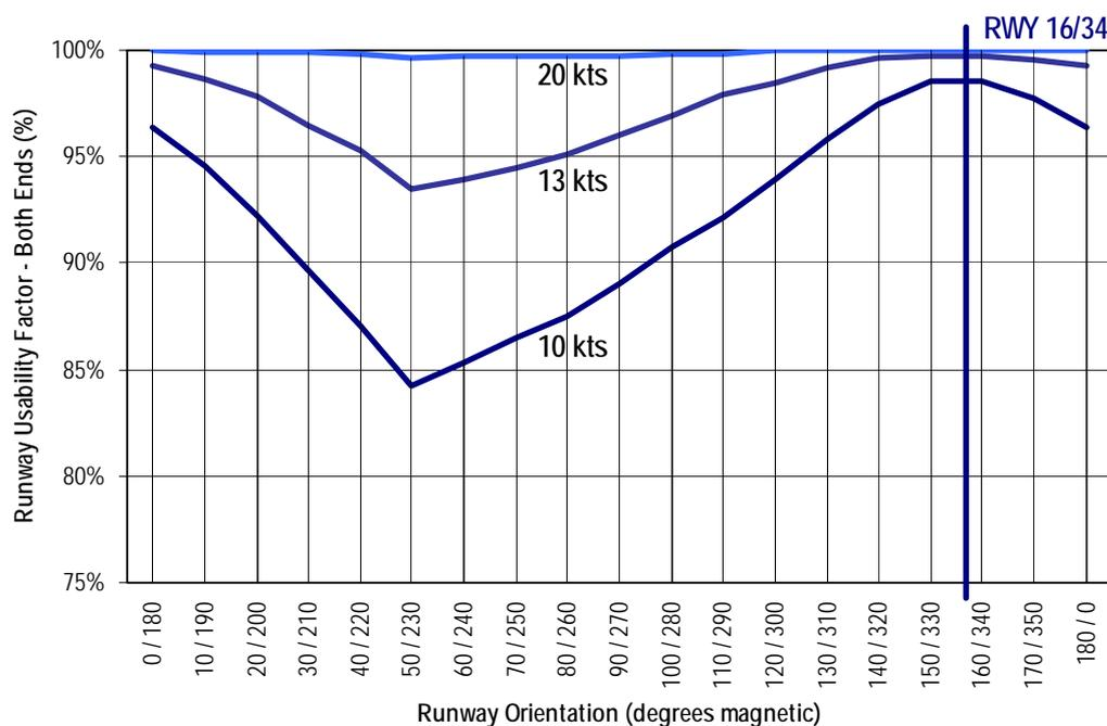
Analysis shows that the optimum direction for a cross runway would be approximately 16/34. However, the overall usability will be maximised if the cross runway is oriented in the range 150-180° Magnetic.
