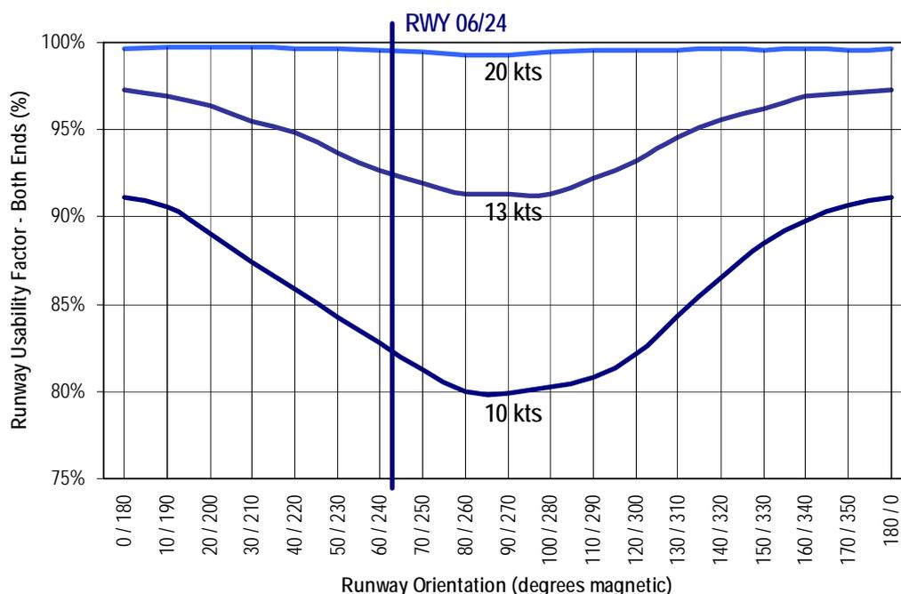
Analysis of wind conditions shows that the optimum runway direction is 03/21 with 21 being the preferred runway. It would provide very close to 100% usability in 20 knot crosswind conditions.
