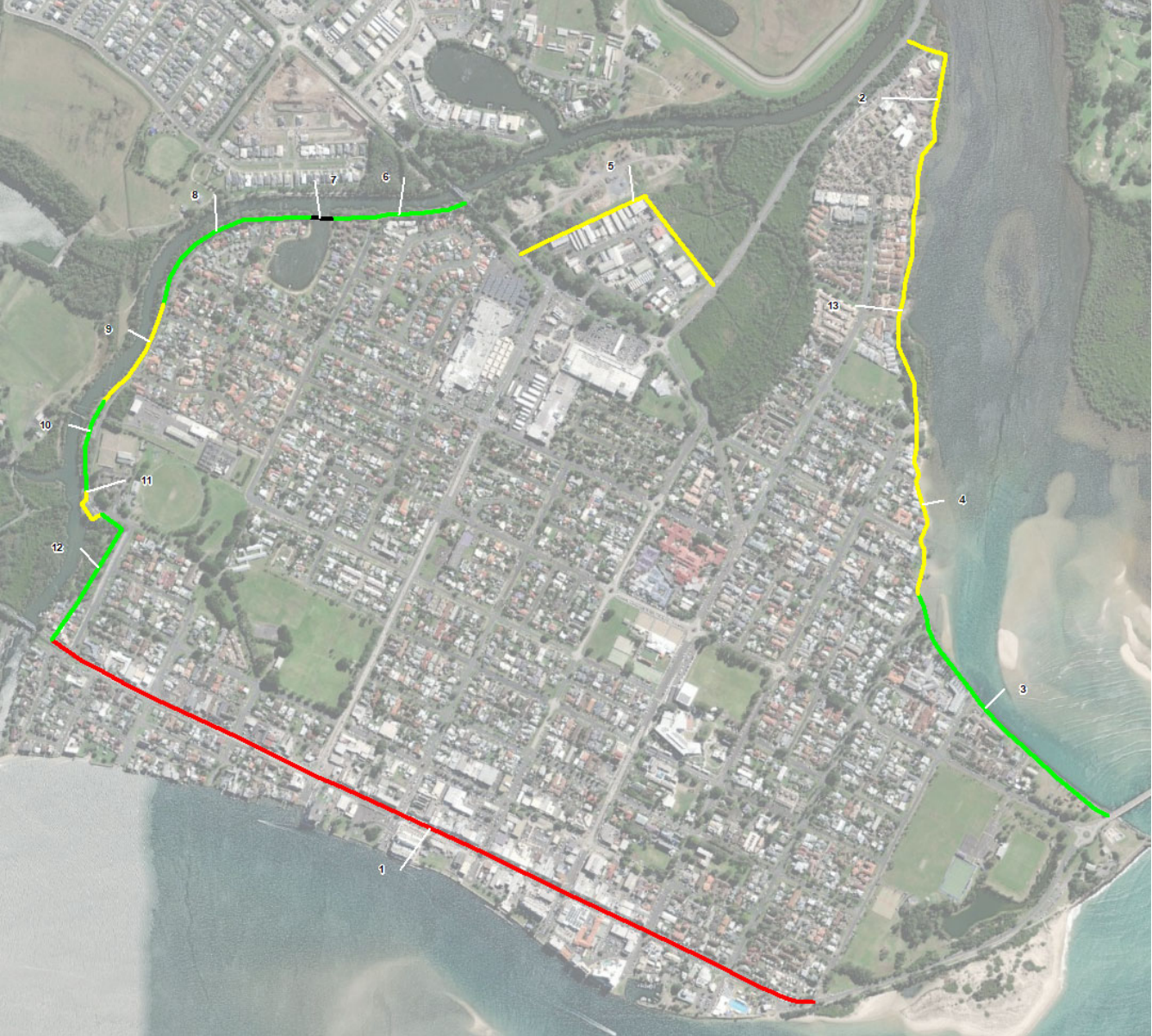
Figure C1. Ballina Island Levee (Levee Sub-Sections 1 to 13)
