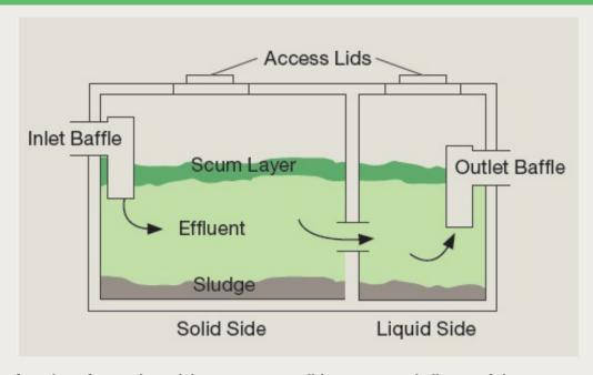
The major function of a septic tank is to separate solids, grease and oils out of the wastewater before it enters the drainage beds/trenches.
