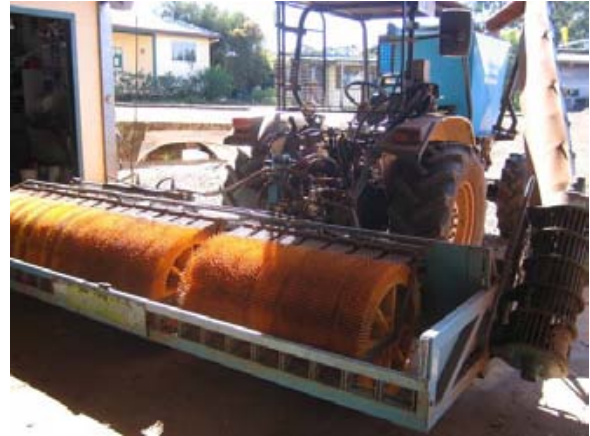
Example of a finger wheel harvester used in the macadamia industry
