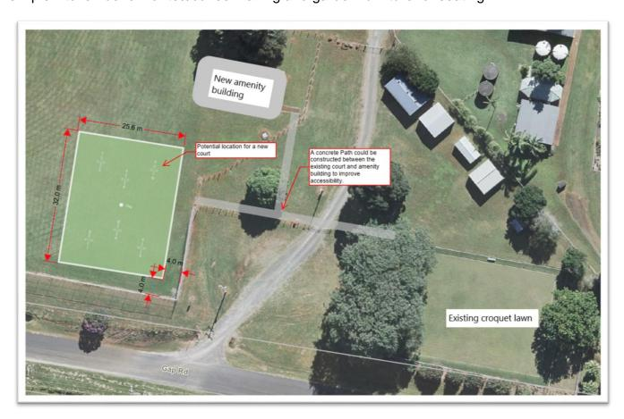
The new amenity building could be constructed over the existing footprint with connection to existing services. A suitable building for croquet could be achieved at ~80m² in size and
