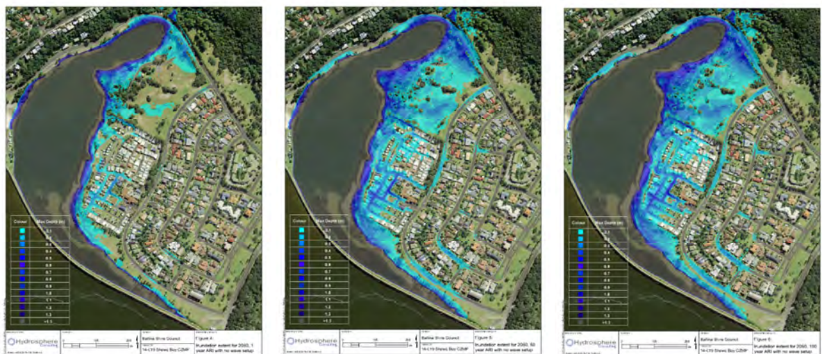
Figure 22: Predicted 2050 inundation due to 1, 50 and 100 year ARI ocean level events (not including wave setup)
